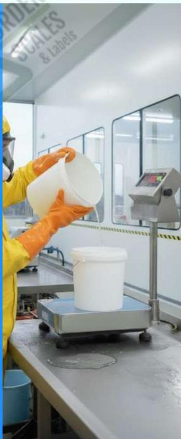
Equipped with the trusted Micro A12E indicator, the scale delivers clear visibility through a bright red LED display, with zero and tare functions for seamless operation. The dual power system — AC mains and rechargeable battery — ensures uninterrupted use, whether on the factory floor or in a mobile setting. Connectivity is built-in too, with RS-232 output for data transfer or printer integration.
