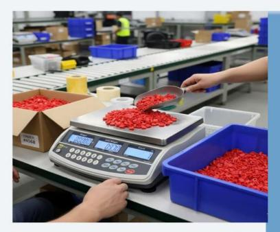
The scale comes equipped with essential functions designed to streamline counting tasks. With features such as piece counting, tare, accumulation, zero tracking, and a configurable quantity alarm, the Micro QHC eliminates guesswork and time-wasting manual counting. It also allows storage of up to 10 product memories, helping speed up repetitive tasks and improving efficiency across your operations.
