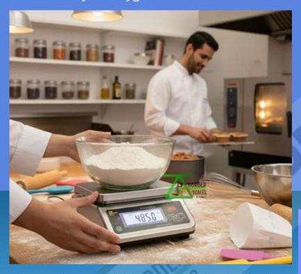
The scale is available in 6kg and 15kg dualrange models, giving users both accuracy and flexibility. The 6kg version provides 1g/ 2g precision, while the 15kg version offers 2g/ 5g precision—ideal for weighing both small ingredients and larger product portions.
